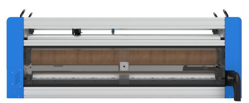
> Transverse pre-cutting machine on **moving film**.
